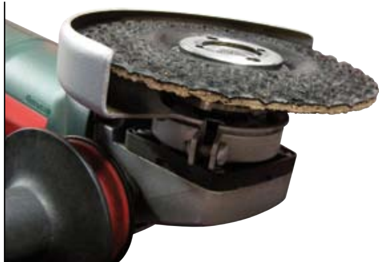
The mounting flange disappears completely into the wheel's cavity.
