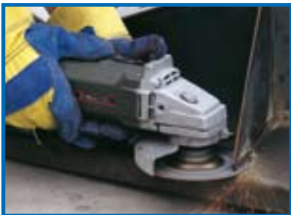
Safecut: horizontal flush cut
